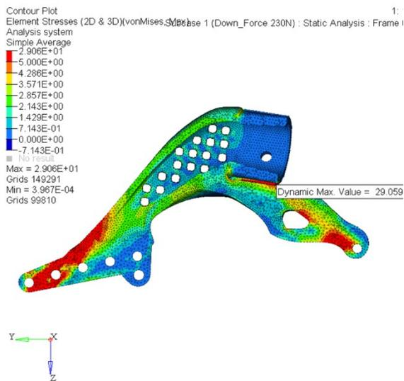
This led to a much lighter version of the metal ALM bracket which weighed just 144gms (was 210gms). A cross section of the model is shown on the left and the hollow section also allows for un-sintered support material to be removed post manufacture.
