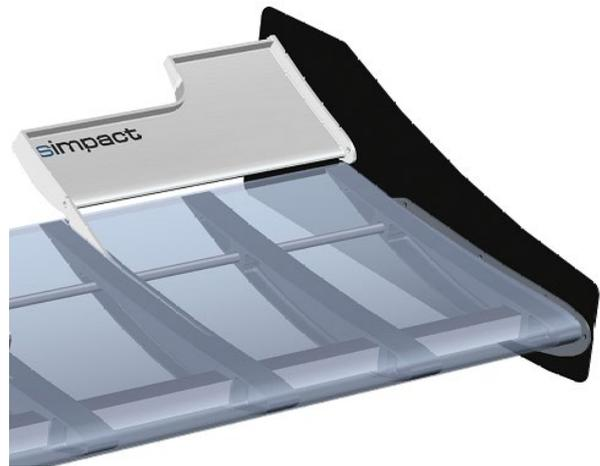
Secondary winglets are 3D printed entirely in ABS where the internal core used a lightweight honeycomb geometry (defined by the 3D printer) for its core. The secondary winglets provide extra downforce and help divert air over the front wheels and are mounted outboard enough not to restrict air into the side pods.
