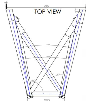
The design made use of existing (off the shelf) butted tubing that Reynolds had in stock. For example, the diagonals (in the top view above) made use of tapered rear chain stay tubes (used to support the rear wheels on bicycles) where the tube thickness is 0.8mm at the top joint and thins down to 0.4mm. Requiring no tooling investment, it is well suited for low volume manufacture. The structure is secured to the chassis using fasteners (for quick disassembly).
