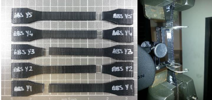
Material property data was applied from existing database and in the case where material properties were unknown samples were made and tensile testing carried out to obtain the relevant material parameters.
