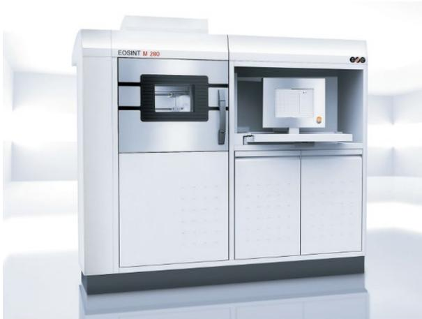
Most people are already aware of the significant advantages that this digital technology brings by being able to produce top quality parts from CAD data fully automatically on very short lead times with no need for any tooling whatsoever. The process builds the parts up layer by layer which enables the creation of extremely complex geometries such as freeform surfaces,
