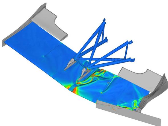
Important target for the impact loadcases was to have sacrificial failure and energy absorption in the wing rather than the supporting nose structure as this is a more economic and desirable scenario.
