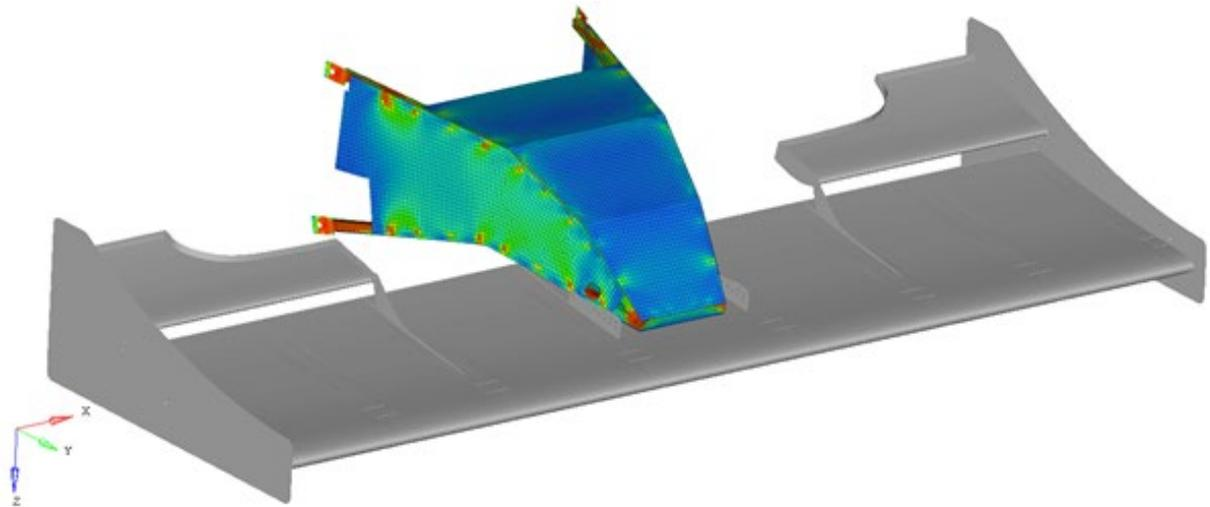
This information and a target setting exercise on the allowable displacements provided the inputs required for a topology optimisation exercise to derive the basic shape of the component of the metal ALM component. The only constraints being the design volume available and the design for the fixation/adjustment. The image below shows the evolution of the design in Optistruct.
