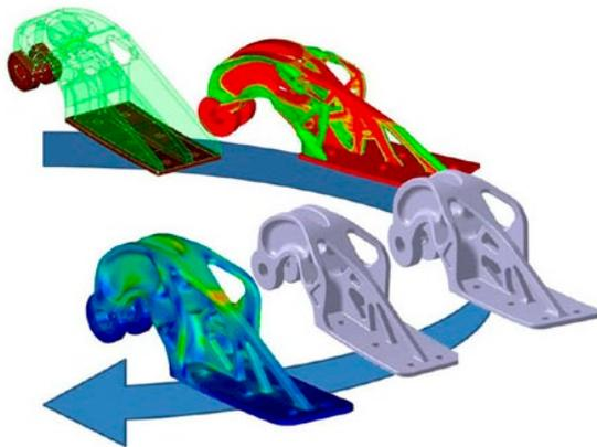
The software of choice for this project was Altair HyperWorks. This includes the Optistruct and RADIOSS software suitable for the analysis of linear and non-linear (crash) loadcases respectively.
