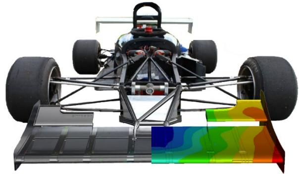
which is a method to analyse the structural response of systems to anticipated loadcases before the part is manufactured. Providing accurate geometry and material properties are available, this approach allows for the development of a highly optimised structure and is eliminates the needs for physical prototypes.
