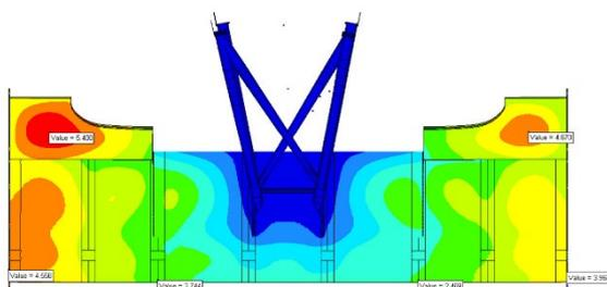
The image on the left shows a displacement contour plot from one of the in-service loadcases (uniformly distributed loading – note the slight asymmetric vertical displacement due to the asymmetric nose frame design)
