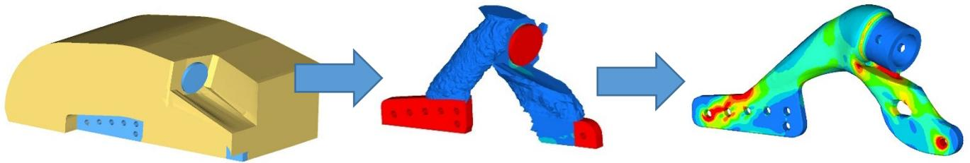
The baseline optimisation drove the v-shaped bracket shown above and the need for a high strength material. Maraging steel was chosen for the sinter material as the EOS data sheet offered very good material properties (2000MPa yield stress) and part accuracy. Although the above derived design was solid in section at this stage of the optimisation, it enabled for the detailed analysis and fine-tuning and weight reduction of the complete system and other wing component assemblies.
