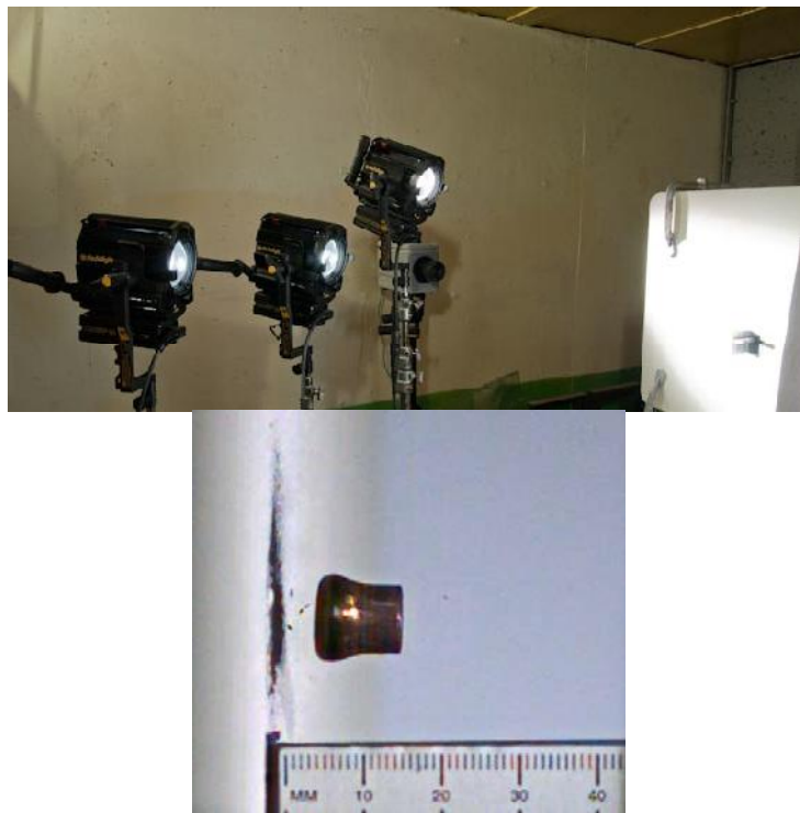
Figure 2. Experimental setup (left): The ballistic target is a flat, hardened steel plate. Three lighting units provide necessary illumination for a High Speed Video (HSV) camera which captures the impact (right).
