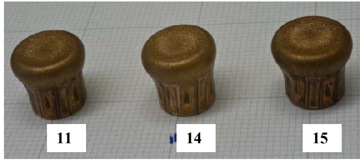
Figure 4. Post-impact bullet heads 11 (116.8 m/s), 14 (116.3 m/s) and 15 (120.8 m/s), GM specification.
