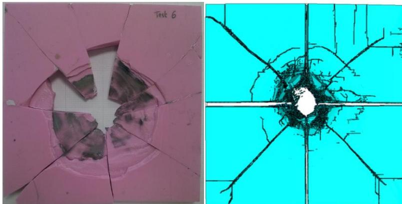
**Figure 10.** Back-to-back comparison between reassembled target and simulation results (Test 6)
