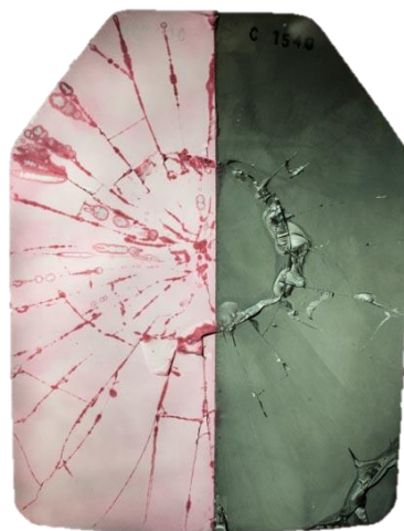
Figure 3. Test armour with visible damage pattern in form of cracks
